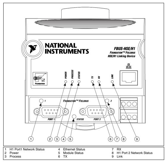
Figure B-1. LEDs on the FBUS-HSE/H1 LD
